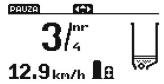
On the screen: number of the current path =3, maximum number of the path (tramline) =4, current speed 12,9 km/h, first cylinder extended, second cylinder in motion, seed level in the container (currently low);
